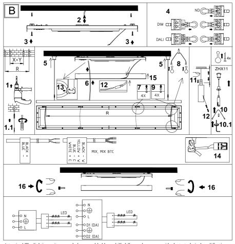
Attention! The lighting unit may only be assembled by a skilled firm or by person with electrotechnical qualification. The light source of this luminaire is not replaceable, when the light source reaches its end of life the whole luminaire should be replaced.
